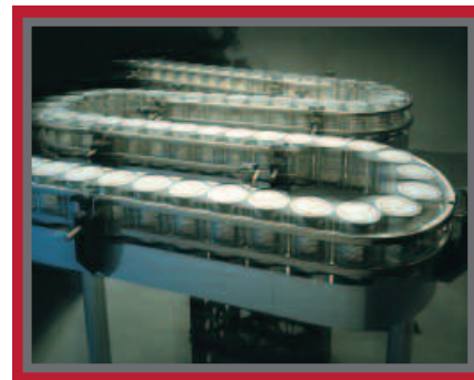
XCS Systems Ltd. designed a project for a canning plant to easily integrate over 160 motors using PowerFlex drives and RSLogix 5000 Software version 16 into a new conveyor line.
